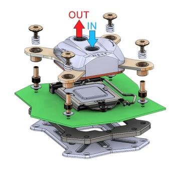
picture. Slide one of the four supplied springs onto each bolt and secure each spring using one of the knurled head screws (only one or two revolutions). Alternately fasten each screw a fraction of a revolution until all four screws are fully fastened.
